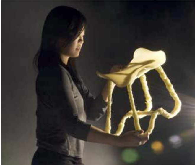
Figure 3: Kim (2011) Milky Chair, experimental material/process using rice, milk and vinegar. Material innovation and application is an inherent part of Design and Craft studies.
