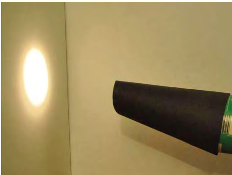
Figure 4: Snoot made from paste paper
