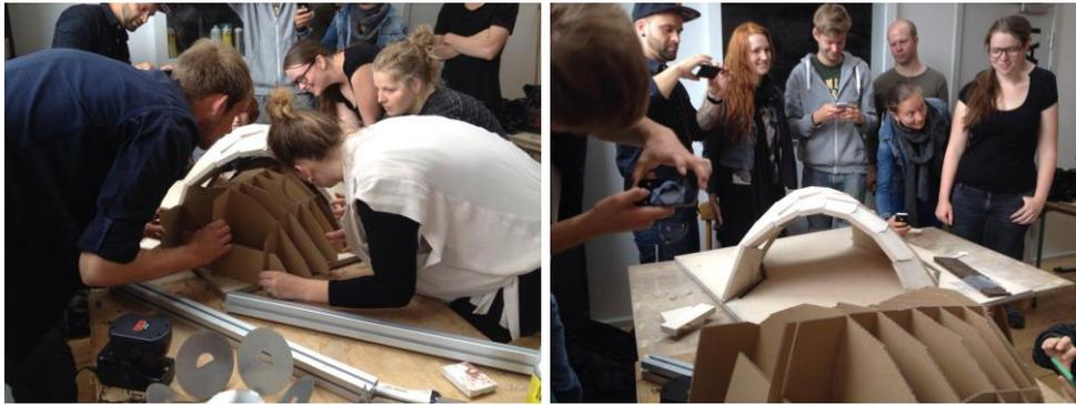
Figure 1: (Left) Centering being removed from the plywood vault. (Right) Free-standing plywood test vault with centering in foreground.
